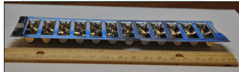
Images from top: Schematic cross section of a CPC integrated with solar cell strips; Prototype CPC array bent around a 2-inch radius; Prototype of 12 CPCs integrated with 30 mm x 2 mm solar cell strips
